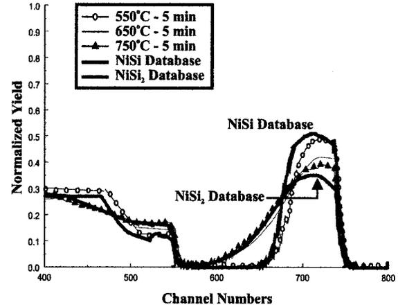
FIG. 6. RBS spectra for 5 min anneals at 550, 650, and 750 °C. Also shown are spectra for samples established as the NiSi and NiSi<sub>2</sub> databases (solid lines).
