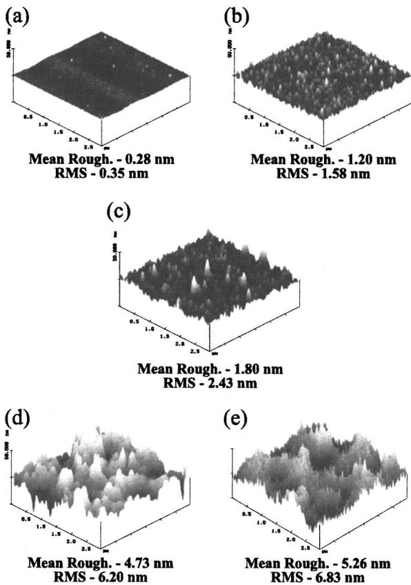
FIG. 2. AFM images, mean and rms roughness values for: (a) Ni on Si, and for samples annealed at (b) 250 °C, (c) 500 °C, (d) 800 °C, and (e) 1000 °C for 30 s.
