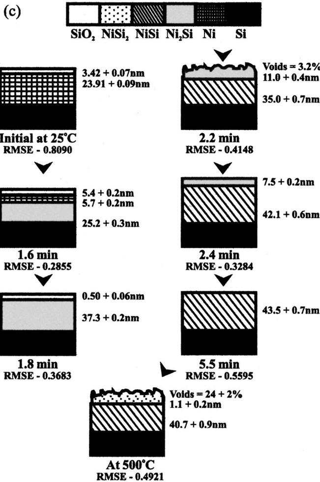
FIG. 10. (a) RTE, (b) SE, and (c) SE models for the temperature ramping stage during annealing from 25 to 500 °C over 11.5 min.
