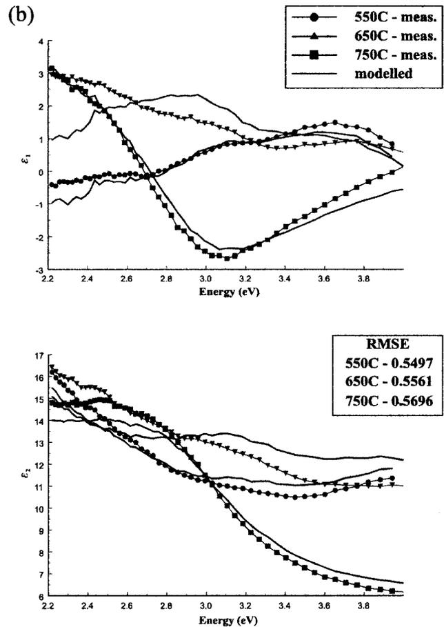
FIG. 8. (a) SE models for short and long time anneals, and (b) model fits for 5 min anneals at 550, 650, and 750 °C. Also shown are the RMSE values for the fits.
