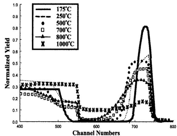
FIG. 1. RBS spectra for 30 s anneals at 175, 250, 500, 700, 800, and 1000 °C.
