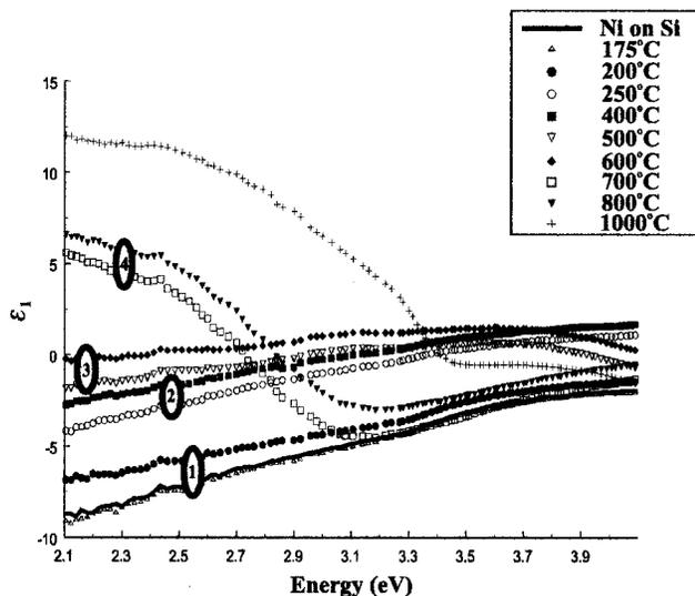
FIG. 4. SE spectra for samples annealed for 30 s. Also marked are four groups of spectra that represent predominantly: (1) Ni on Si, (2) Ni<sub>2</sub>Si, (3) NiSi, and (4) NiSi<sub>2</sub>.
