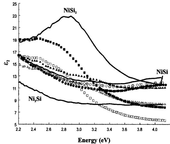
FIG. 7. SE spectra for samples annealed for longer times at 550, 650, and 750 °C. Also shown are the nickel silicide databases (solid lines).
