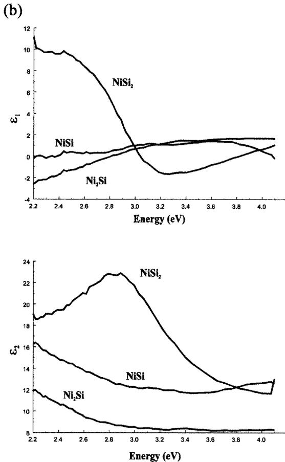
FIG. 5. (a) Ellipsometric models, and (b) SE spectra for the nickel silicides established as databases.
