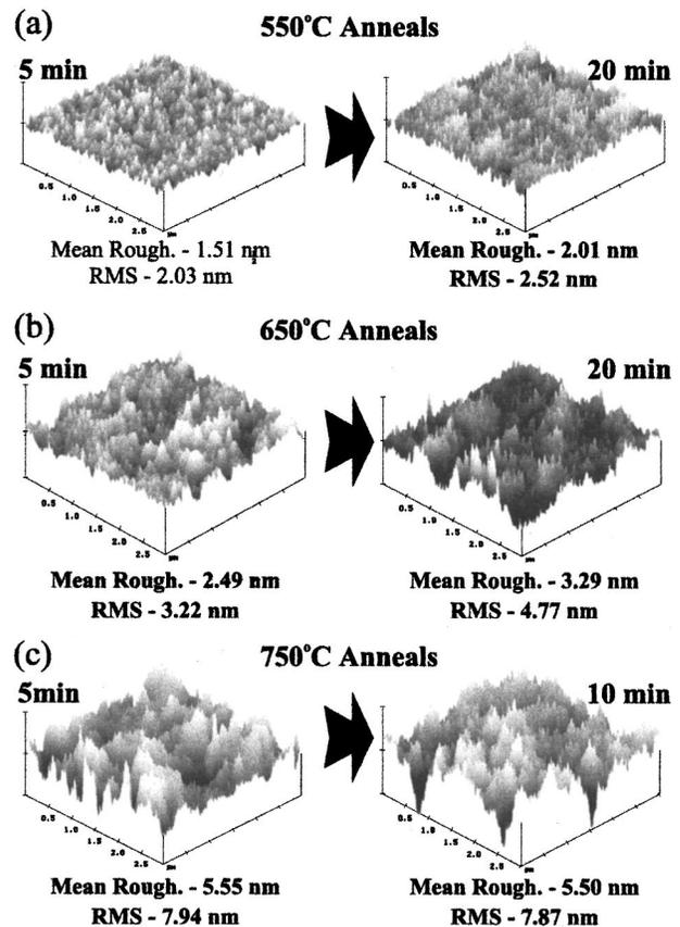
FIG. 3. AFM images, mean and rms roughness values for samples annealed at: (a) 550 °C, (b) 650 °C, and (c) 750 °C for longer times (5, 10, or 20 min as specified).
