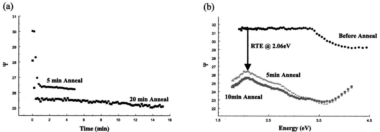
FIG. 9. (a) Single wavelength real-time, and (b) spectroscopic ellipsometry data for anneals at 550 °C for 5 and 20 min in the RTP system. RTE data taken at 2.1 eV.
