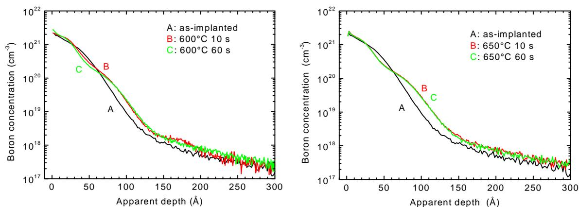
**Figure 1:** SIMS profiles of 500 eV boron, implanted to a dose of  $1 \cdot 10^{15} \text{ cm}^{-2}$ , and after  $600^\circ\text{C}$  or  $650^\circ\text{C}$  for 10 s or 60 s annealing in pure argon gaseous ambient. **Left:** B:  $405.55 \Omega/\square$ , C:  $785.7 \Omega/\square$ ; **Right:** B:  $784.62 \Omega/\square$ , C:  $797.64 \Omega/\square$
