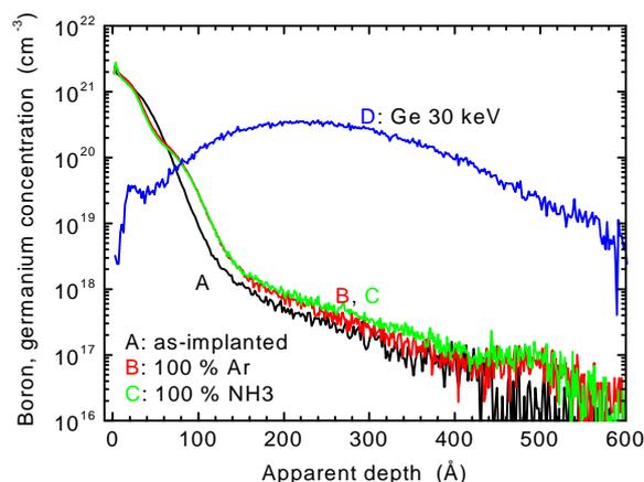
**Figure 4:** SIMS profiles of the as-implanted and subsequent SPEG boron annealed distributions in a 30 keV germanium pre-amorphised Si layer. ( $^{11}\text{B}^+$ , 500 eV,  $1.0 \cdot 10^{15} \text{ cm}^{-2}$ ) to demonstrate the dependence of the SPER on the gaseous ambient for constant thermal budget ( $650^\circ\text{C}$  10 s). The sheet resistance values are as follows. B:  $784.62 \Omega/\square$  (100 % Ar), C:  $826.45 \Omega/\square$  (100 %  $\text{NH}_3$ ).
