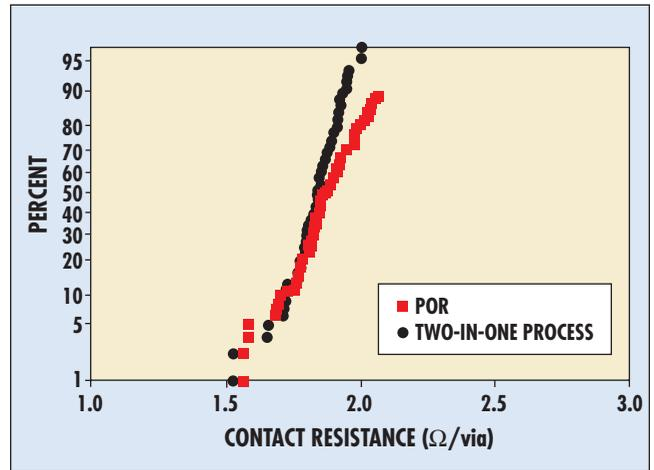
Figure 8: Normalized probability chart showing via-chain resistance.
