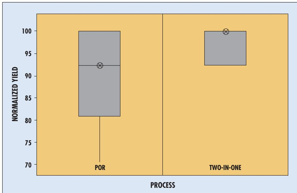
Figure 9: Normalized probability chart showing via-chain yield.
