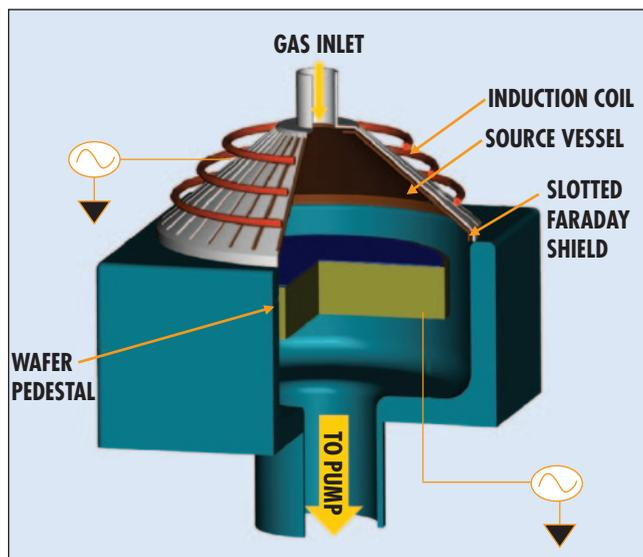
**Figure 3: Plasma source and stripping station of the two-in-one system.**
