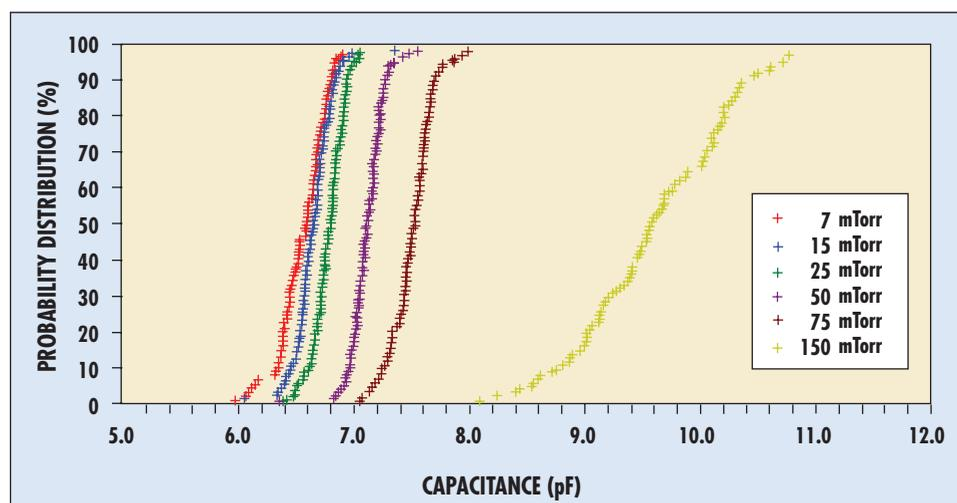
**Figure 1: The 0.25/0.30- $\mu\text{m}$  comb capacitance test results from MSQ films showing dependence of RC product on process pressure.**
