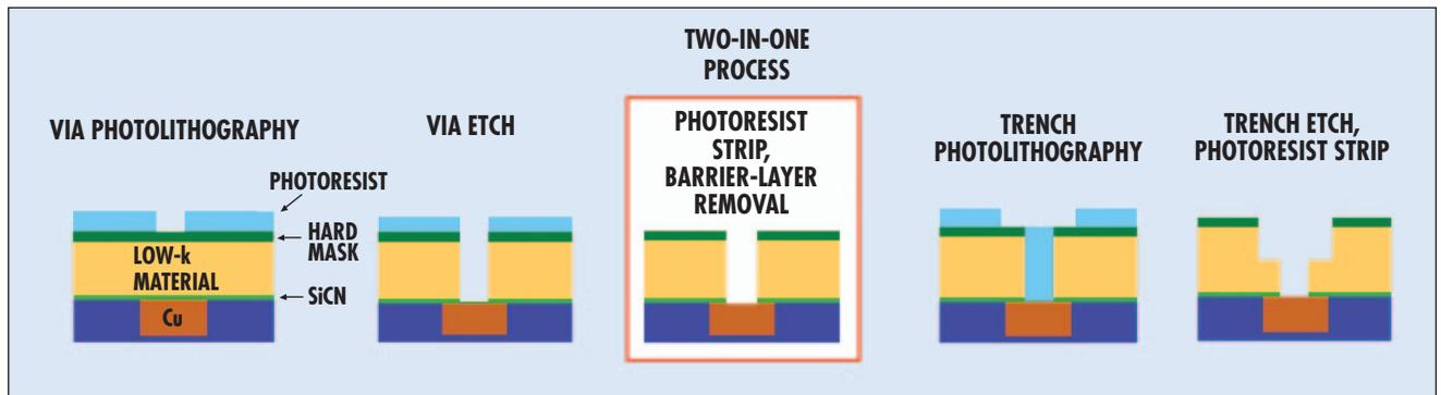
Figure 2: Schematic diagram showing system integration scheme of the two-in-one process.
