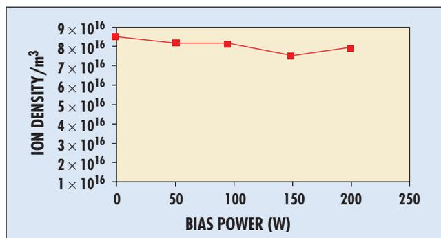
Figure 6: Measured ion density versus bias power in the two-in-one system.
