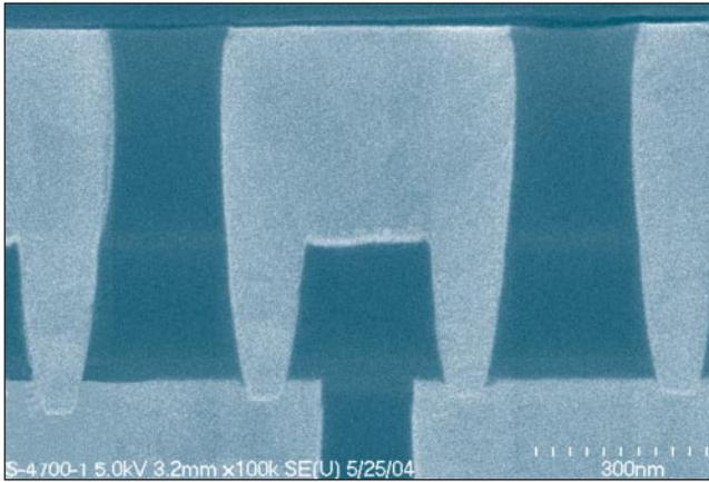
**Figure 10: Cross-section SEM image of a copper/low-k interconnect structure manufactured using the two-in-one process.**
