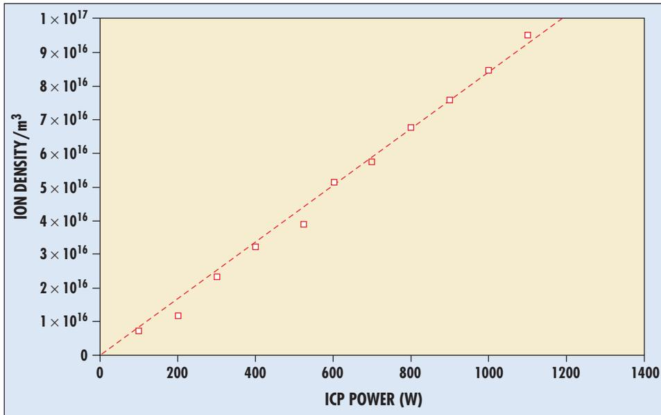
Figure 5: Linearity between ion density and inductively coupled power.
