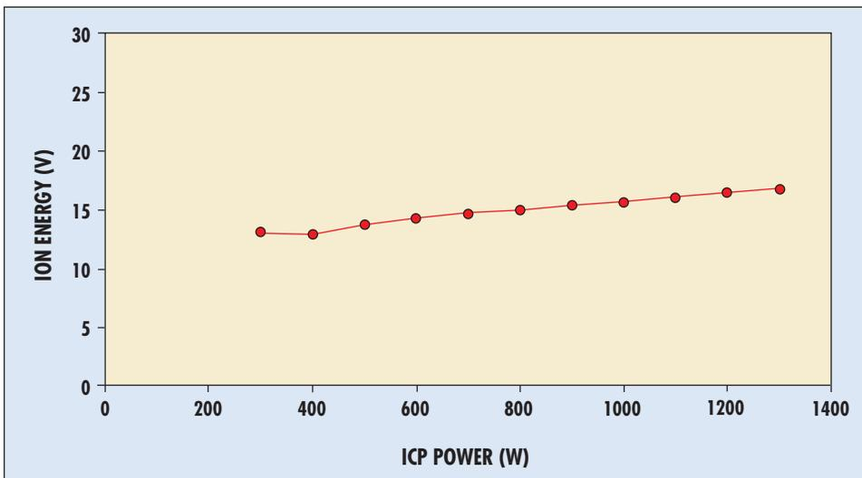
**Figure 4: Dependence of plasma potential on ICP power.**
