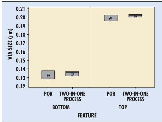
Figure 7: Electrical test results for via bottom and top CD.
