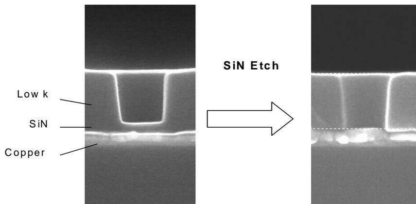
Fig.6 Process performance of copper barrier removal.
