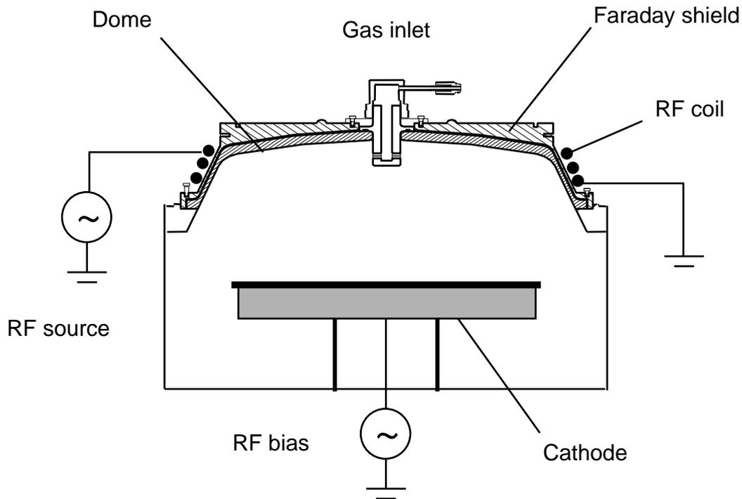
Fig.1 Schematic diagram of Highlands plasma reactor.
