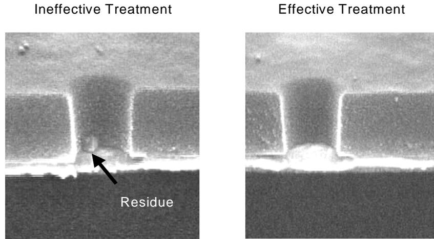
Fig.7 Comparison of effective and ineffective copper treatment.
