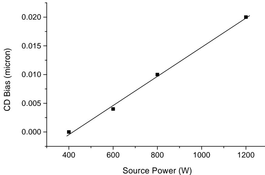
Fig.5 Source power dependence of CD bias after barrier removal.
