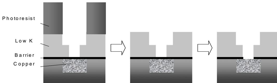
Fig.2 Process flow of 3-in-1 process integration.
