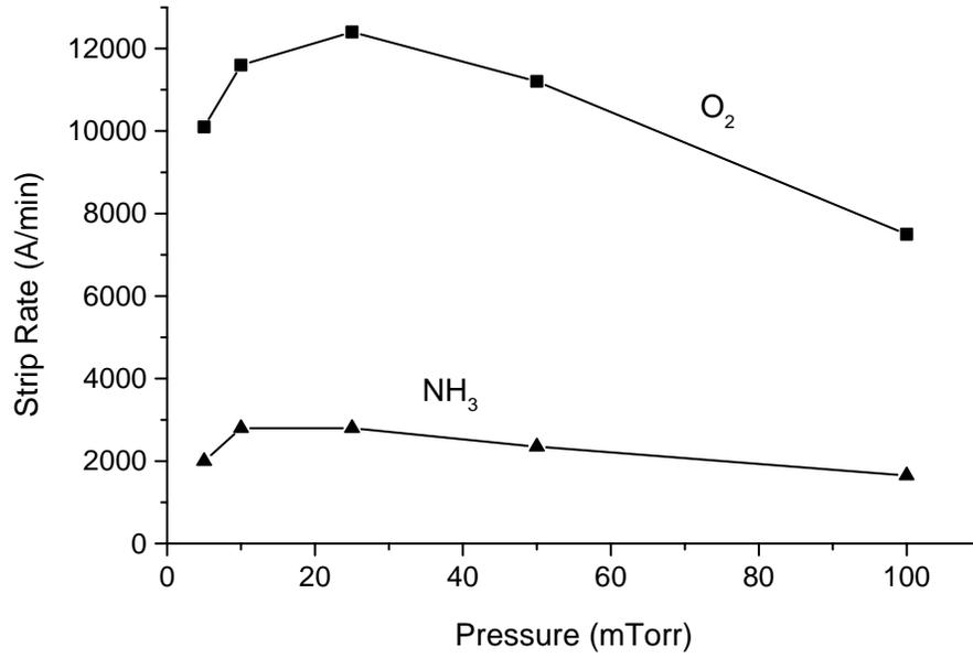
Fig.3 Dependence of photoresist strip rate on pressure.
