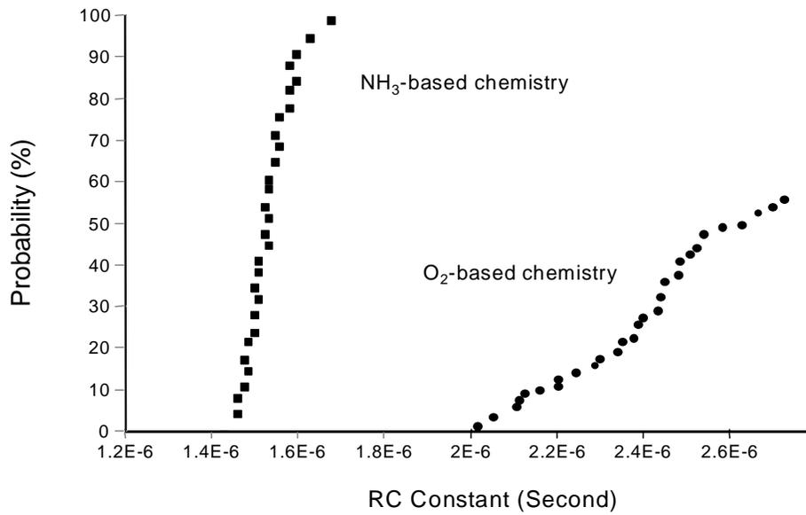
Fig.4 Effect of photoresist strip chemistry on RC constant.
