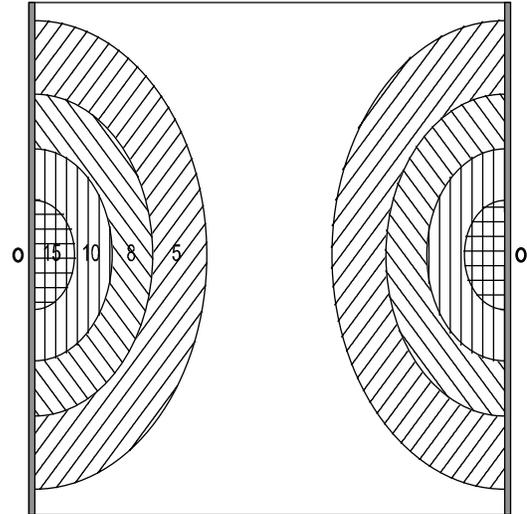
FIGURE 2. Contour map showing the magnitude of the peak induction electric field in the ICP source. The field varies radially inwards from a maximum of 15 V/cm to 5 V/cm and in both directions axially from the center turn of the induction coil.
