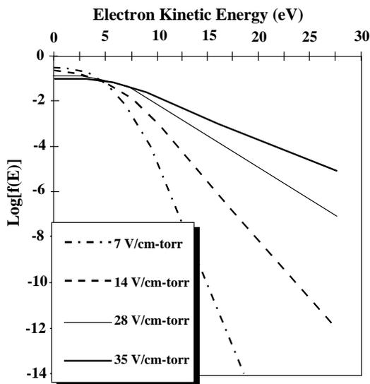
**FIGURE 3.** The electron energy distribution function calculated for different values of E/N, the induction electric field divided by the gas pressure (V/cm-torr).
