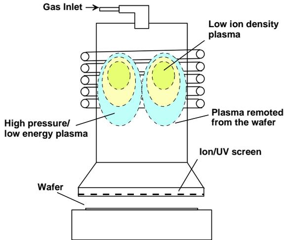
The magnetic field reverses direction at 13.56 MHz, the frequency of the rf generator, resulting in a very rapid periodic change in the magnetic flux parallel to the cylinder axis. This changing flux induces a circumferential electric field which is parallel to the walls of the cylinder. The equation which governs the induction electric field is given by
